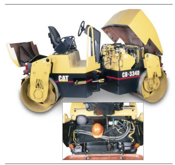
**Engine enclosure** pivots upward and locks into place.
