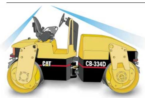
**Excellent forward visibility** allows the operator to see objects 0.6 m high and 1 m in front of the machine.
