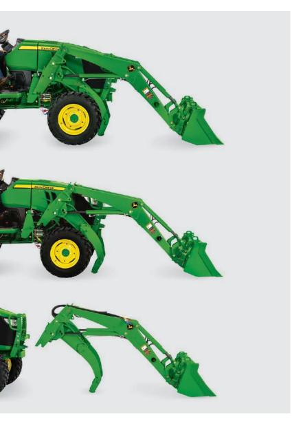
**Quik-Park™ loader mounting system:** H and R Series loaders are designed for easy, tool-free mounting and removal. The parking stand is attached to the front frame of the tractor and becomes an integral part of the loader during loader operation. To drop the loader to the 'park' position, just lift the joystick after opening the latches.
